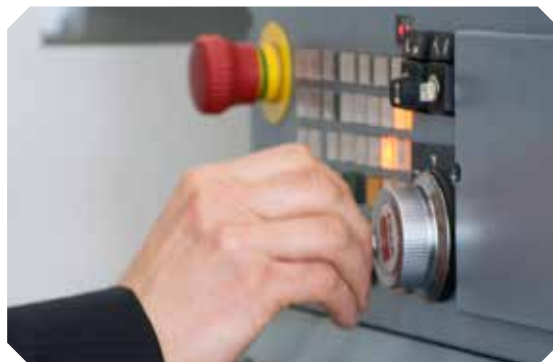
Use of the hand-wheel to translate the whole tool path
