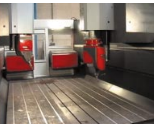
Boxer 418: the simultaneous use of bi-swivelling milling heads
